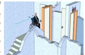
minimum distance of 9 m between the two exits would qualify these to be remote exits.
